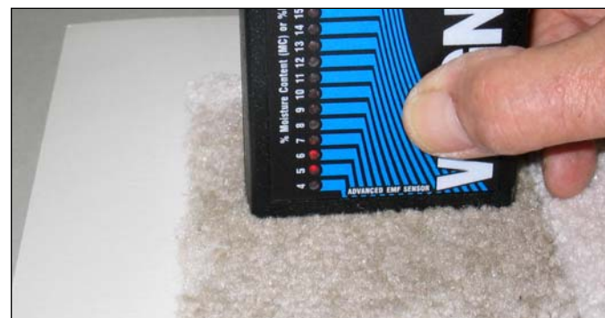
PHOTO 8 – TESTING FOR DRYING
