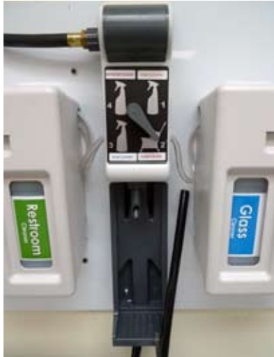
Lockable cabinets and auto dilution eliminates chemical contact
